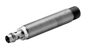
Inductive Proximity Sensor, 3-Wire DC, Short Barrel, 18mm Diameter, Tubular:Nickel Plated Brass, Short, 8mm Sensing Distance, Unshielded, N.O., Source (PNP) Output, Micro QD (DC)
