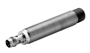
Inductive Proximity Sensor, 3-Wire DC, Short Barrel, 18mm Diameter, Tubular:Nickel Plated Brass, Short, 5mm Sensing Distance, Shielded, N.O., Source (PNP) Output, Micro QD (DC)
