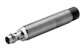
Inductive Proximity Sensor, 3-Wire DC Standard Barrel, 8mm Diameter, Tubular:Nickel Plated Brass, 2mm Sensing Distance, Shielded, N.O., Source (PNP) Output, PVC Cable (5 Cond)
