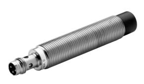
8mm Cylindrical Nickel-Plated Brass Inductive Proximity Sensor, 3-Wire DC, 2mm Sensing Distance, Shielded, N.O., NPN/PNP Selectable, 4-pin M12 DC Micro QD
