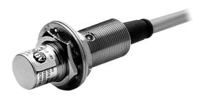
Inductive Proximity Sensor, 3-Wire DC Extended Range Standard Barrel, 30mm Diameter, Unshielded, Tubular:Stainless Steel, Metal Face, 40mm Sensing Distance, N.O., Source (PNP) Output, Micro QD (DC)
