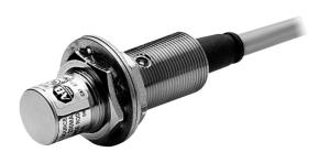
Inductive Proximity Sensor, 3-Wire DC Standard Barrel, 18mm Diameter, Unshielded, Tubular:Stainless Steel, Metal Face, 8mm Sensing Distance, N.O., Source (PNP) Output, Micro QD (DC)
