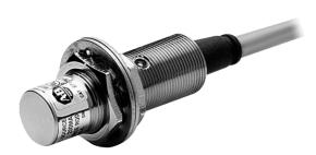
Inductive Proximity Sensor, 2-Wire AC/DC (PLC Interfacer), 18mm Diameter, Unshielded, Tubular:Stainless Steel, Metal Face, 8mm Sensing Distance, N.O. Output, ToughLink Cable
