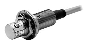
Inductive Proximity Sensor, 2-Wire AC/DC, 18mm Diameter, Shielded, Tubular:Stainless Steel, Metal Face, 5mm Sensing Distance, N.O. Output, PVC Cable
