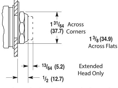
Bootless Flush and Extended Head Momentary Contact Push Button Shipping Weight. 5-1/2 oz (0.16 kg) Dimension Diagram
