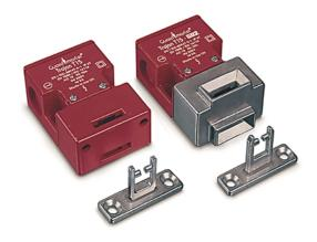
Tongue Switch - Trojan T15: Contacts(Safety and Aux): 1 Normally Closed, 1 Normally Open, BBM Preference: N/A, Actuator: No Actuator, Model Type: GD2 Front Entry, Conduit Entry: M20 Conduit
