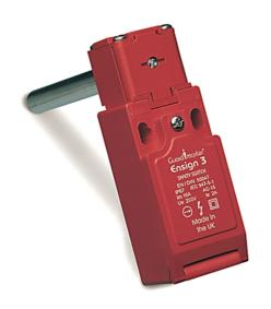
Hinge Switch - Ensign 3: Contacts: (Safety/Aux) 2 Normally Closed / 1 Normally Closed, BBM Preference: Break Before Make, Actuator Shaft: Length: 80MM Diameter: 10MM-Solid, Conduit Entry: M16 Conduit
