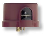
¬ Electronic type with a conventional positive switching ratio. These devices use an integrated chip together with a silicon light-sensing element and maintain specification performance levels for up to five times longer than conventional cadmium sulphide (CdS) controls. The combination of these design features prevents light level drift so that the light switching levels remain constant for the life of the control unit.
