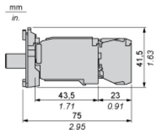
Plug-in Connector, Integral LED
