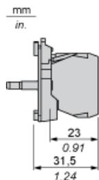
Screw Clamp Terminal Connections, Direct supply for BA9s Bulb
