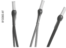
Triple probe to be inserted into equipment
