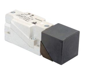
IC Series Inductive Proximity Sensors, thermoplastic polyester housing 40\*40\*118mm, 20 to 250 V AC/V DC power supply, Power MOSFET NO output, 30mm sensing range, IP67 rating, fully protected, LED-indication for power and output ON
