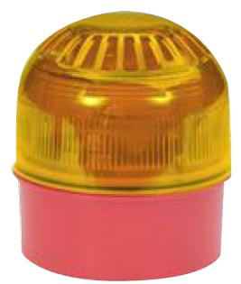
Sonos Electronic Sounder, Red base with Amber LED beacon on top, 17-60V DC, 32 tones, dB range 93-106, IP65
