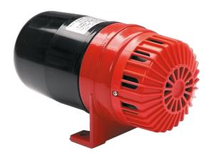
Mono 72, Motor driven siren 110V AC, IP65, 1800 Hz, 120dB @ 1 metre  $\,$
