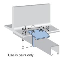
Suits P1000 & P2000 Design Load Per Pair: 4.32kN Finishes: Z.P. & H.D.G. Mass: 49kg/100
