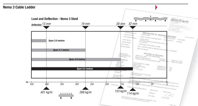
Nema 3 Cable Ladder has been tested in accordance with the Nema requirements by a NATA certified testing facility. The data displayed is based on physical test results of a 600 wide section and may vary for other widths. The Deflections have been provided as a guide based on continuous spans, and cannot be applied to end spans. Data provided assumes that the installation will be carried out in accordance with Nema VE2, non compliance may affect the overall product performance.
