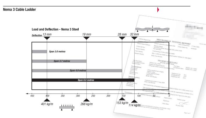
Nema 3 Cable Ladder has been tested in accordance with the Nema requirements by a NATA certified testing facility. The data displayed is based on physical test results of a 600 wide section and may vary for other widths. The Deflections have been provided as a guide based on continuous spans, and cannot be applied to end spans. Data provided assumes that the installation will be carried out in accordance with Nema VE2, non compliance may affect the overall product performance.
