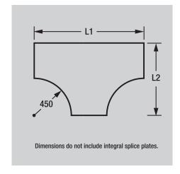
Order fasteners separately for installation. 12 x Splice Bolts (SBH) & 12 x Splice Nuts (SNH) required.
