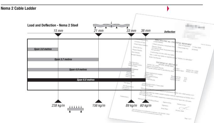
Nema 2 Cable Ladder has been tested in accordance with the Nema requirements by a NATA certified testing facility. The data displayed is based on physical test-results of a 600 wide section and may vary for other widths. The Deflections have been provided as a guide based on continuous spans, and cannot be applied to end spans. Data provided assumes that the installation will be carried out in accordance with Nema VE2, non compliance may affect the overall product performance.
