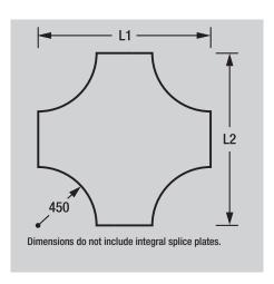
Order fasteners separately for installation. 16 x Splice Bolts (SBH) & 16 x Splice Nuts (SNH) required.
