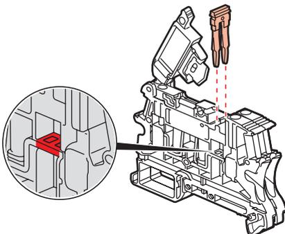
The combs remain visible when the handle lever is closed, and remain accessible when the mini lever is closed.
