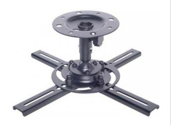
Designed to suit a majority of projector models in the market today. All steel ball mount bracket allows up to 30° of adjustment either vertically or horizontally which is more than enough for more installations! The projector mounting surface sits 115mm from the ceiling and may be removed from the upper bracket for adjusting the projector settings if required. Two sets of mounting arms are provided (140mm &180mm) and may be adjusted on the base plate as desired.
