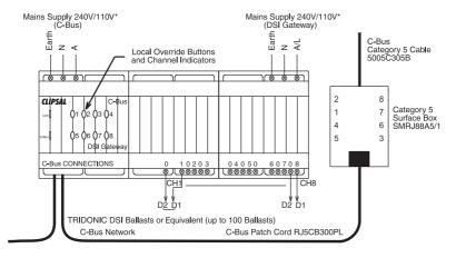
\* For 5508DSIP use 240V~, 50/60Hz and for E5508TDSIP use 110V~, 50/60Hz
