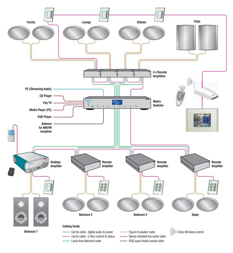
\*This System Overview is a 'typical' 8 zone C-Bus Multi-Room Audio system. A C-Bus Multi-Room Audio system can start with a single zone and expand to 24 zones depending on user requirements. Please contact Clipsal for further information.
