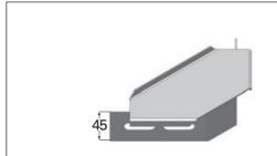
2 TX Brackets required to make a tee, and 4 required to make a cross. Order fasteners separately for installation (per TX Bracket)
