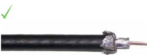
Fold back the first braid then fold back the first foil. Fold back the second braid but DO NOT remove the last foil as this is bonded to the Dielectric. Fold back braid and foil evenly in each direction to ensure the connector slides on easily. A good preparation should look like the following diagram.
