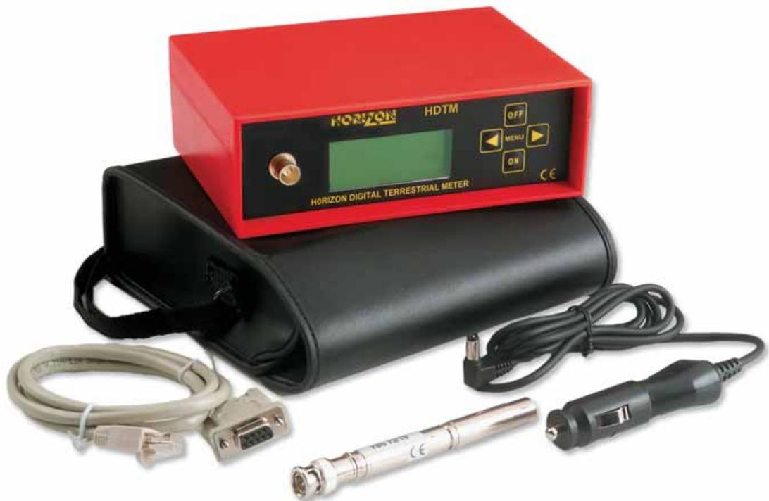
This meter is a Digital Field Strength Meter and will not measure any channel below VHF 6.
