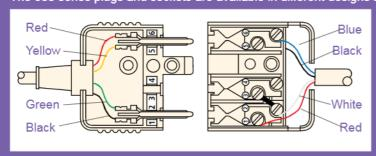
Cable Colour CodingPairTip (L+)Ring (L-)1WhiteBlue2RedBlack3OrangeGreen
